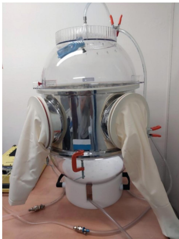
Figure 2. The sealed chamber developed based on NIOSH guidelines (NIOSH 2016).
